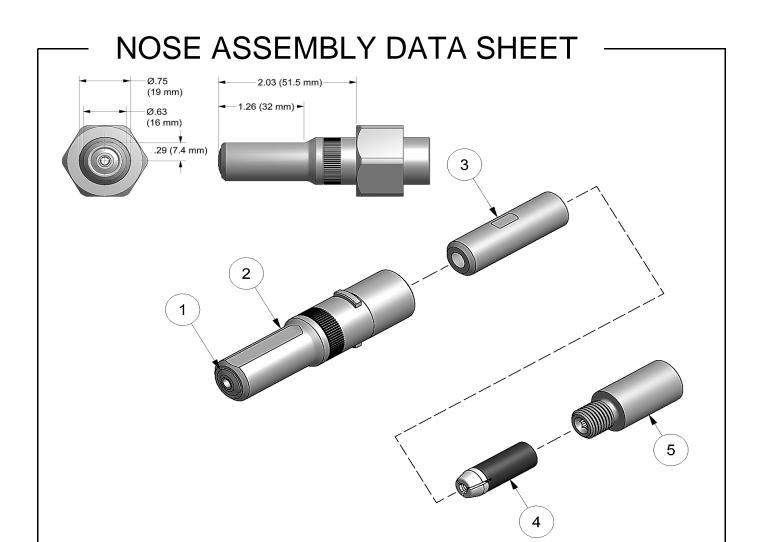
Use Hex-Key in rear of piston for nose assembly attachment.
