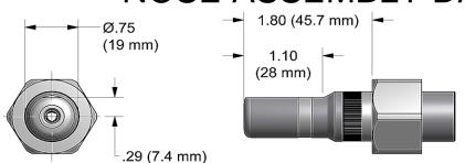
Use Hex-Key in rear of piston for nose assembly attachment.
