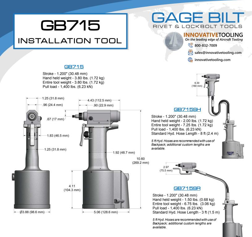
The GB715 series are pneumatic-hydraulic tools designed specifically for the efficient installation of blind rivets. They can be operated in any position. They have a rated pull load of 1,400 pounds (6.23 kN) with 90 psi (6.2 bar) air pressure at the air inlet.
